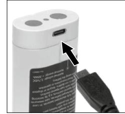
! The battery may **only** be charged with the battery charger provided and used only in **this** laser device. Any other use may cause injury or fire.
