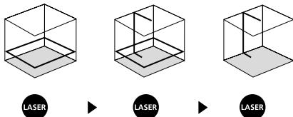
**!** The transport restraint must be released for horizontal and vertical levelling. The laser lines flash when the device is outside the automatic levelling range of 3°. Position the device such that it is within the levelling range.
