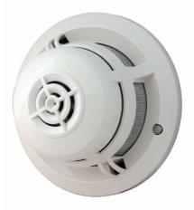
The ESMI 2251CTLE-W plug-in fire detector combines 4 separate sensing elements to act as a single unit. CO sensing for monitoring CO products from a smouldering fire, IR sensing for measuring ambient light levels and flame signatures, optical smoke detection and heat detection.
