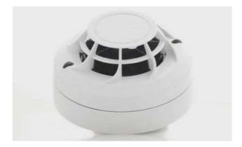
The ESMI 52051E and ESMI 52051HTE are fixed temperature analogue addressable sensors employing low mass thermistors and microprocessor technology for fast response and linear temperature sensing. Their linear response allows these sensors to be used to signal temperatures over the range of 58℃ (Class A1S) to 78℃ (Class BS).
