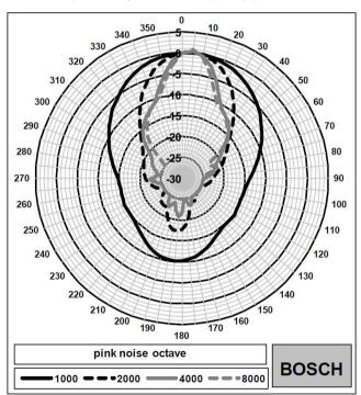
Horizontal polar diagram (high frequency part)
