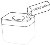
2 Remove the upper cover and fill the water tank;
