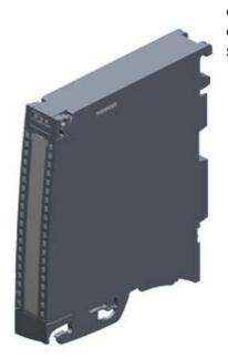
SIMATIC S7-1500, ANALOG OUTPUT MODULE AQ 2 X U/I ST, 16 BITS OF RESOLUTION, ACCURACY 0.3 %. 2 CHANNELS IN GROUPS OF 2, DIAGNOSIS, SUBSTITUTE VALUE INCL. FRONT CONNECTOR PUSH-IN, FEEDING ELEM., SHIELDING ELEM., SHIELDING CLAMP
