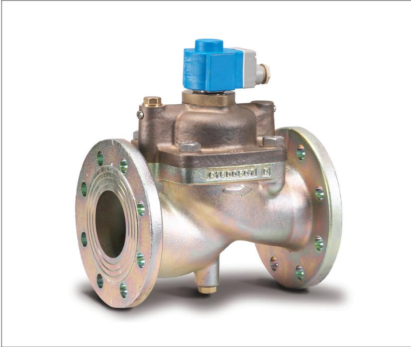
EV220B 65 - EV220B 100 is a 2/2-way solenoid valve program for use in robust industrial applications, demanding high flow rates. The valve is designed with cast iron valve body and flanged connection. Water-hammer damped design and built-in pilot filter ensures a reliable operation.
