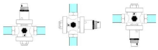
The pressure reducers EUROBRASS 143 don't get the effects, in their functioning, of gravity force; therefore they can be installed in the plant in any position:
