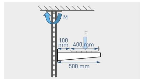
1: Calculation of force on the bracket - F
