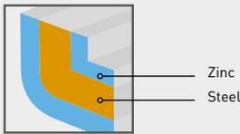
The steel (iron) is protected with a layer of zinc
