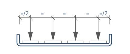
NB: In the case of short brackets with side fixings (CAT30, CM50, etc) the maximum deflection is measured at the end of the system.
