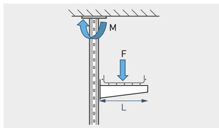
1: Calculation of force on the bracket - F.
