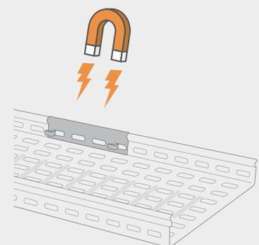
The metal structure of the cable tray absorbs some of the electromagnetic disturbance and converts it into noise current.
