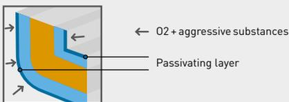
In the open air, zinc self-passivates which leads to a matte appearance, and can create a thin white film on the part.
