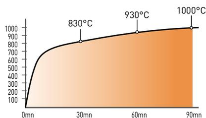
The approval awarded (E90, E60, E30) is obtained for a predefined span and load. The validation criterion for fire resistance systems is defined by whether the electrical equipment still works when it comes out of the furnace. For an approved configuration, the cables and cable trays see their mechanical properties definitely altered but they have fulfilled their purpose: to ensure the installation lasts for a defined period.
