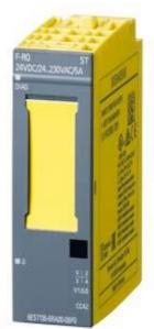
SIPLUS ET 200SP F-RQ 24 V DC/24-230 V AC/5 A -25...+60°C start up -25°C with conformal coating based on 6ES7136-6RA00-0BF0 . F-RQ 1x 24 V DC/24..230V AC/5A ST, 20 mm overall width, 1 relay output (2 NO) Summation output current 5 A, load voltage 24 V DC and 24.. 230 V AC, Can be used up to PL E (ISO 13849-1: 2008)/ SIL 3 (IEC 61508: 2010) if control takes place by (e.g. 6AG1136-6DB00-2CA0) F-DQ
