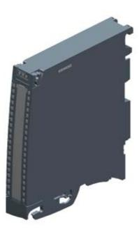
SIMATIC S7-1500, DIGITAL OUTPUT MODULE, DQ 16 X 24VDC/0.5A; 16 CHANNELS IN GROUPS OF 8, 4 A PER GROUP; INCL. FRONT CONNECTOR PUSH-IN
