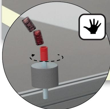
The Threaded Collor (M8/M12) is mounted onto the Rubber Damper prior to installation on to the Heat Pump.
