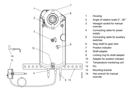
Arrangement for shaft adapters
