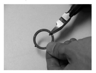
3.12 Install the ring over the cable and dummy rod.
