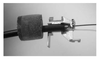
3.5 Tighten the screw to fix the strength member.
