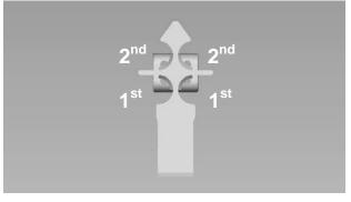
3.4 Position the cable onto the cable bracket and fit in the strength member as shown.
