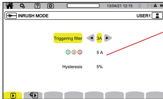
The threshold takes into account the current present, in order to detect the appearance of an additional current.
