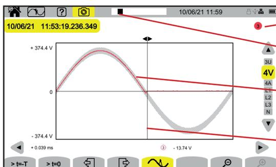
Reminder of the number of the channel that triggered the transient capture.
