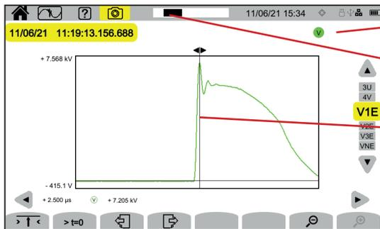
Reminder of the channel that triggered the shock wave capture.
