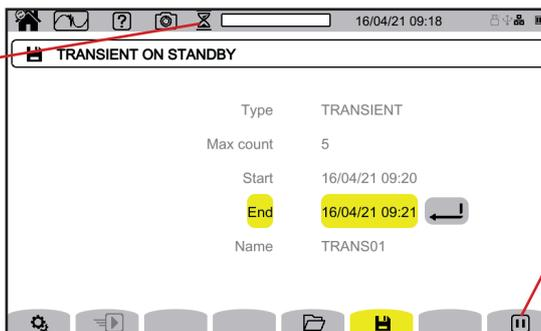
To suspend the recording in progress.
