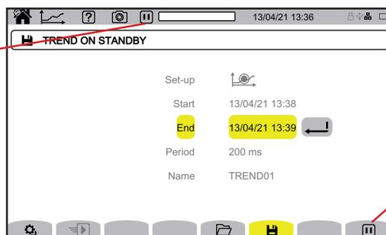
To suspend the recording in progress.
