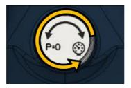
The measuring system should be vented after a few seconds. Close the bypass again to measure. Turn the rotary knob clockwise in the direction of the "Pressure Measurement" symbol:
