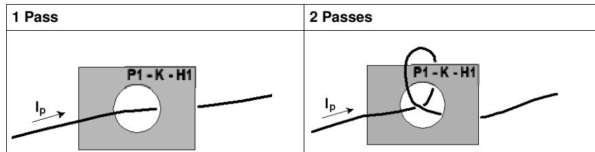
All three CTs must be connected in the same way in order to ensure **identical relative polarity**: the cable must be routed in the same direction for the three current transformers (entering via the side marked P1-K-H1).
