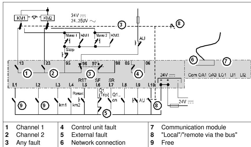
**NOTE:** To feed back external data via the communication bus (write to a register) using inputs I.1 and I.2, operation must be configured in "**remote via the bus**" mode. (Refer to the documentation for the communication module)
