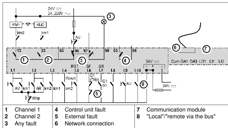
3-wire control with local operation, "remote via the bus" operating mode and data feedback (voltage local control > 24 V).
