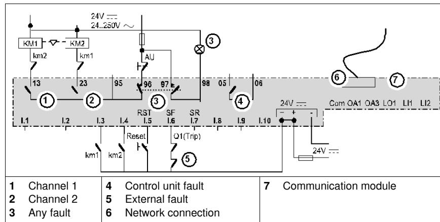
**NOTE:** To feed back external data via the communication bus (write to a register) using inputs I.1 and I.2, operation must be configured in "**remote via the bus**" mode. (Refer to the documentation for the communication module)
