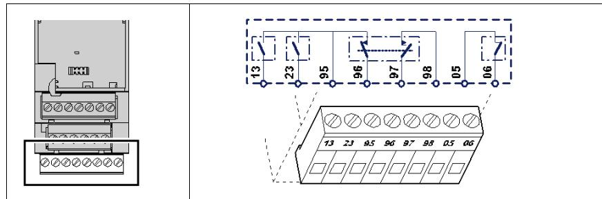
**NOTE:** The contacts (95 - 96) and (97 - 98) are shown with the controller powered up, input I.6 at 1 and in the absence of any fault condition.
