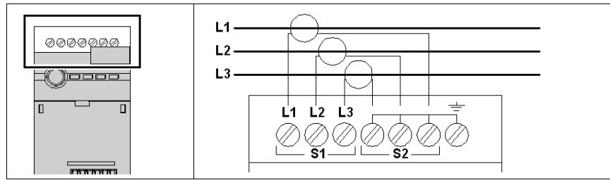
These terminals can be used to measure the current in all three phases:
