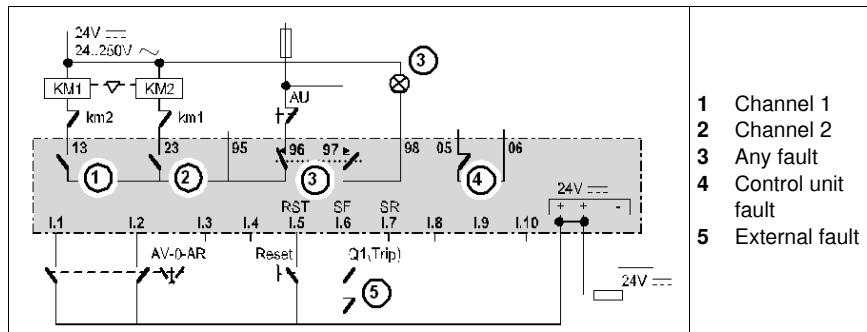
3-wire control by the controller I/O (reversing)
