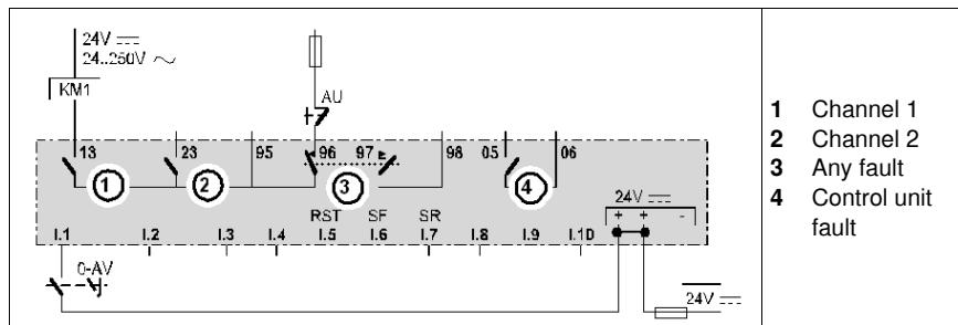
2-wire control by the controller I/O (reversing)
