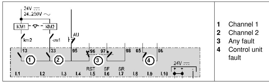
There is no longer a fault contact in series with the contactor coils.
