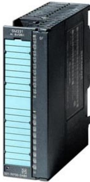
SIMATIC S7-300, ANALOG INPUT SM 331, GALVANICALLY ISOLATED, 8 AI, 14 BIT, 0.052MS/CHANNEL, CURRENT, VOLTAGE, INTERRUPTS, DIAGNOSTICS, 1 X 20 PIN, FIT FOR ISOCHRONOUS MODE IMPROVED DP-CYCLE TIME FOR ISOCHRONOUS MODE
