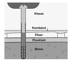
**4.** The balancing effect of the flexible edge strip.
