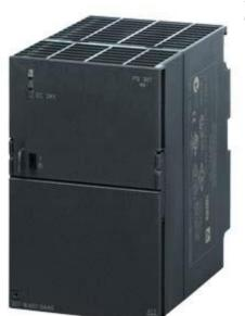
SIPLUS S7-300 PS 307 10A -25 ... +70 DEGREES C WITH CONFORMAL COATING BASED ON 6ES7307-1KA02-0AA0 . STABILIZED POWER SUPPLY PS307 INPUT: 120/230 V AC OUTPUT: 24 V DC/10 A
