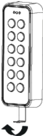
4. When the front of the reader is disconnected from the snap lock, lift the front and slide upwards to disengage from the hook at the top.
