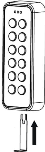
3. Use the opening tool to pull the reader outwards and upwards.
