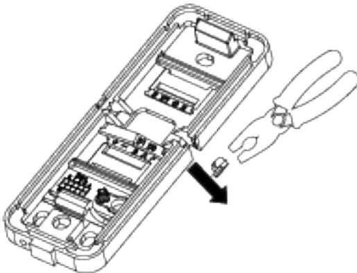
4. Remove the corresponding knockout on the cover.
