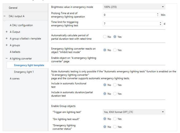
The basic settings for the individual emergency lighting converters and the settings for their tests are made in this window. In addition, group objects to start the test and feed back the result can be parametrized with various codes, again by individual converter. These objects are alternatives to the addressed group objects parametrized in the A lighting converter parameter window. The function is redundant.
