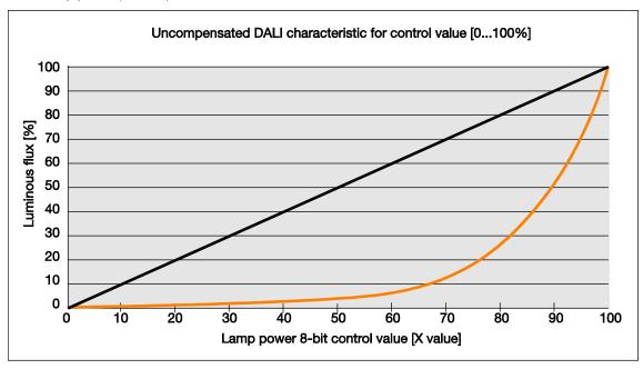
The KNX brightness value received by the gateway is mapped directly to the lamp power. The logarithmic dimming curve calculates the DALI value, so that for the KNX there is linear mapping between the KNX value and the lamp power.
