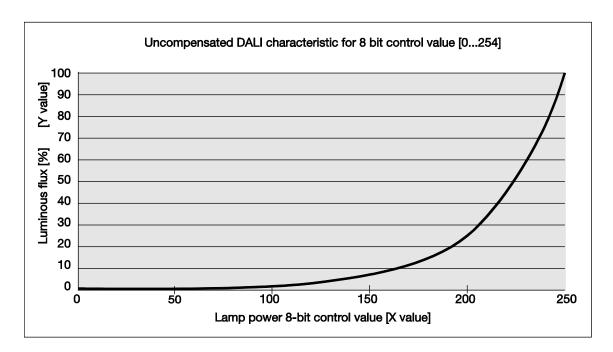
If a DALI (logarithmic) dimming curve is selected in the gateway, the KNX value relates to the 8-bit lamp power control value, the X value.
