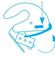
Press the catch again and insert the metal foot back into the handle until it **clicks**. Check that the foot is correctly inserted.
