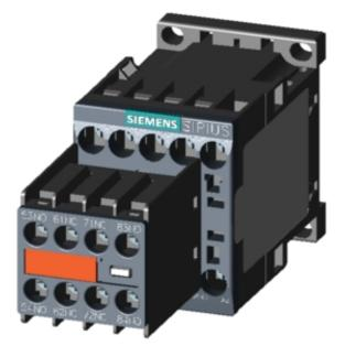
CONTACTOR RELAY, 6NO+2NC, AC 230V, 50/60 HZ, SIZE S00, SCREW TERMINAL, PERMANENT AUX. SWITCH, FOR SUVA APPLICATIONS
