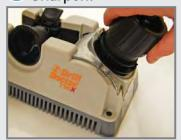
Insert the chuck into the sharpening port and rotate one half turn in a clockwise direction repeatedly until the drill bit is sharp.
