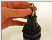
Insert the drill bit into the chuck jaws & tighten the chuck just to the point where the bit can only just slide in and out.
