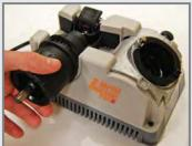
While holding the alignment button down, insert the chuck and slide the drill bit forward until it touches the drill stop. Tighten the chuck firmly.
