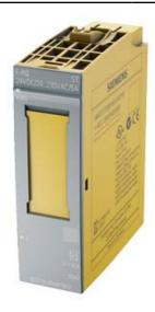
SIMATIC DP, ELECTRON. MODULE FOR ET200SP, F-RQ 1X24VDC/24..230VAC/5A ST, 20MM WIDTH, 1 RELAY OUTPUT (2 NO-CONTACTS) TOTAL OUTPUT CURRENT 5A, RATED VOLTAGE DC 24V AND AC 24 .. 230V, USEABLE UP TO PL E (ISO13849-1: 2008)/ SIL 3 (IEC61508: 2010) IF CONTROLLED BY A F-DQ (E.G. 6ES7136-6DB00-0CA0)
