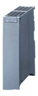
SIPLUS S7-1500 CM PTP RS422/485 -40 ... +70 DEGREES C WITH CONFORMASL COATING BASED ON 6ES7541-1AB00-0AB0 . COMMUNICATION MODUL FOR SERIAL CONNECTION RS422, RS485, FREEPORT, 3964(R), USS, MODBUS RTU MASTER, SLAVE, 115200 KBIT/S, 15-PIN SUB-D FEMALE CONNECTOR
