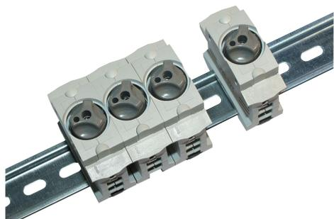
INNOZED® is a fuse base for DO fuse-links, sizes D01 and D02. It is designed for a fast mounting on DIN-rail in distribution boards and panels, for residential and industrial applications.
