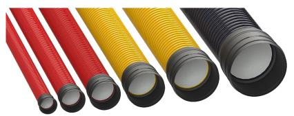
**EVOCAB SUPERHARD N 1250** reinforced double-wall cable protection pipes are designed for underground high-voltage cable lines. Corrugated outer wall ensures high compression strength properties and smooth inner surface of the pipe ensures easy pulling of cables. Due to their special structural properties, these cable protection pipes are lighter, but more rigid, as well as more impact-resistant than the conventional smooth-wall pipes.
