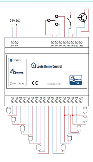
ZIF5020 must be connected to a DC power supply on the terminals marked with 0V and Vin. The power supply must be dimensioned to be able to source the loads connected to the outputs of the module. For example, if it is connected to 10 pieces of 24V 2W actuator on the outputs, then the power supply should at least be able to supply:
