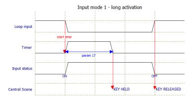
The figure above shows how the timing works at a long activation, where the activation must be longer than the time specified in configuration parameter 13 to be accepted as a long activation (Central Scene Key Held).
