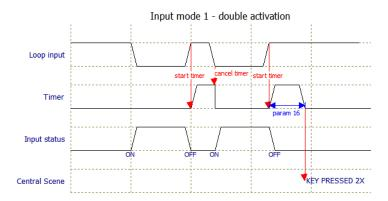
The figure above shows how a double activation is detected. The two activations must happen within the time specified in configuration parameter 12 to be accepted as a double activation.
