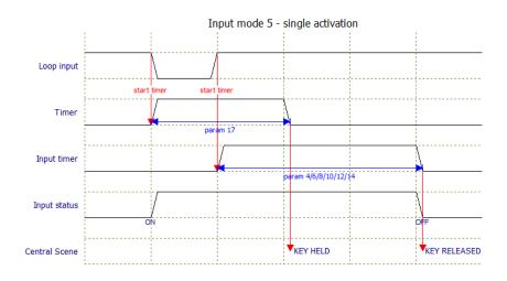
As seen from the above, a KEY HELD Central Scene notification will appear even though the activation on the input is shorter than configuration parameter 17. This is because the status on the input is prolonged with the time specified in the configuration parameter for the input timer (parameter 4/6/8/10).
