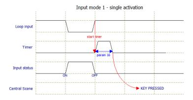
Loop input: Physical signals on the input. Will become 0V when the input is shorted by e.g. a contact.
