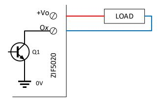
The internal MOS-FET located in the ZIF5020 module can handle a maximum of 60V 1A, but ZIF5020 is "only" sized to be able to supply the module's supply voltage, and a maximum of 1A in <u>total</u> on the + **Vo** terminals (or 0.125A from each of the 8 + **Vo** Maximum 1A total).
