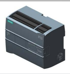
SIMATIC S7-1200F, CPU 1215 FC, COMPACT CPU, DC/DC/RELAY, 2 PROFINET PORT, ONBOARD I/O: 14 DI 24V DC; 10 DO RELAY 2A, 2 AI 0-10V DC, 2 AO 0-20MA DC, POWER SUPPLY: DC 20.4 - 28.8 V DC, PROGRAM/DATA MEMORY 150 KB
