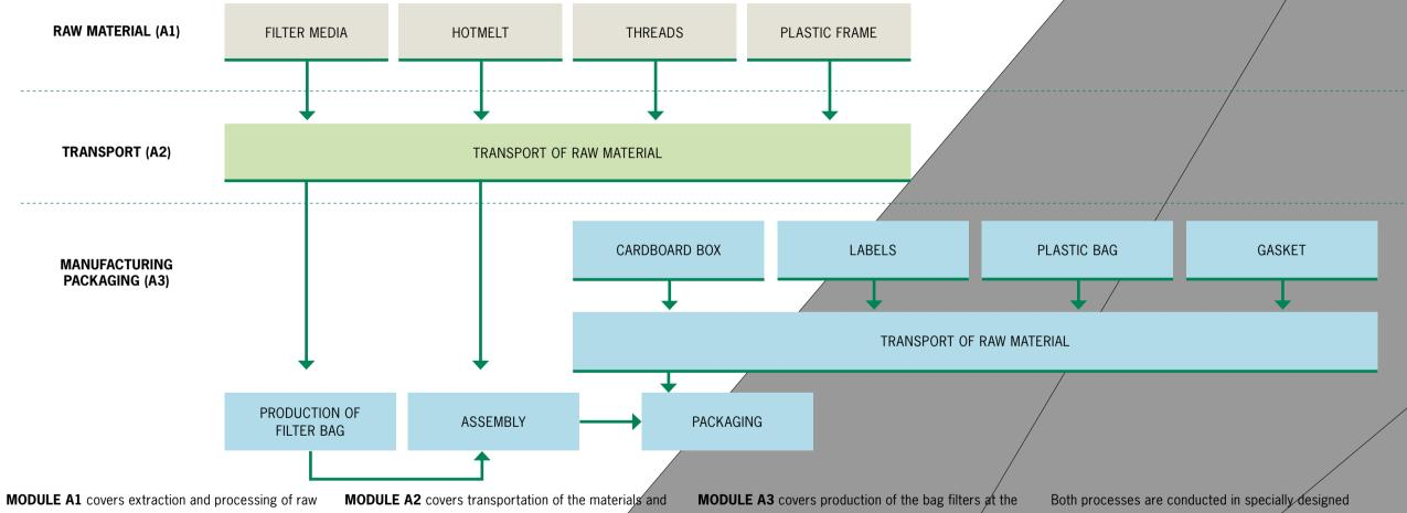
materials, as well as production of the materials and components used for production of bag filters: filter media, plastic frame, hotmelt and threads.
