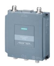
IWLAN Access Point, SCALANCE WAM766-1, 1 radio, 2.4/5 GHz, IEEE 802.11ax (Wi-Fi 6), 2 N-Connect connections, iFeatures support via CLP, 1201 Mbps (gross) per radio, 1x 10/100/1000 Mbps M12 socket, redundant 24 V DC, M12 L-coded , PoE, IP65, -30...+60 °C, CLP slot, DI/DO, A-coded, observe national approvals! CERT ID: MSAX65-W1-M12-E2, FCC ID: LYHMSAX65V1 operation outside of USA/Israel scope of delivery: sealing caps for connections
