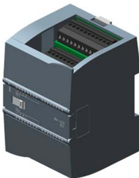
SIMATIC S7-1200, DIGITAL OUTPUT SM 1222, 8 DO, RELAY CHANGEOVER CONTACT
