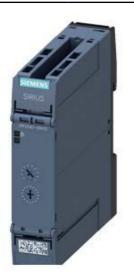
TIMING RELAY, ELECTRONIC, OFF-DELAY, WITHOUT CONTROL SIGNAL OR NON-VOLATILE RELAY DEFINITE PASSING MAKE CONTACT, 7 T. SET. RANGES 0.05...600S, AC/DC 12-240 V, AT 50/60HZ AC, 2 CO CONTACTS, W. LED, SPRING-TYPE (PUSH-IN) TERMINAL
