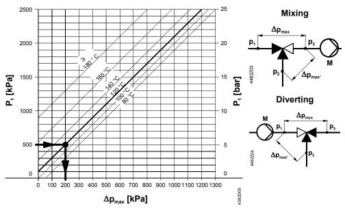
$\Delta p_{max}$  = Differential pressure with valve almost closed, at which cavitation can largely be
