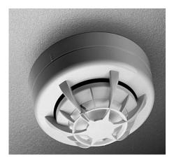
The optical sensor is identical to the one in the Conventia optical smoke detector. Its sensitivity is, however, influenced by a heat sensing element which makes the detector more responsive to fast-burning, flaming fires.
