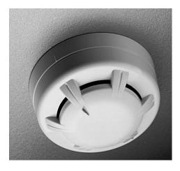
Conventia operates on the well established light scatter principle. The remarkable optical design of the Conventia optical smoke detector allows it to respond to a wide spectrum of fires. The sensing chamber of the Conventia optical smoke detector contains an optical sensor which measures back-scattered light as well as the more usual forward-scattered light. Sensitivity to black smoke is greatly improved.
