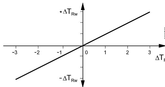
The flow temperature setpoint change  $\Delta T_{Vw}$  resulting from the change of room temperature setpoint is calculated as follows:
