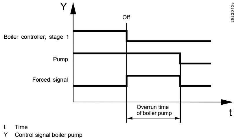
If the boiler sets the forced signal to zero, the consumers and heat exchanges that had responded to the forced signal act as follows:
