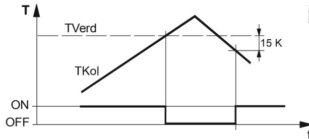
$T_{Verd}$  Evaporation temperature of heat conducting medium
