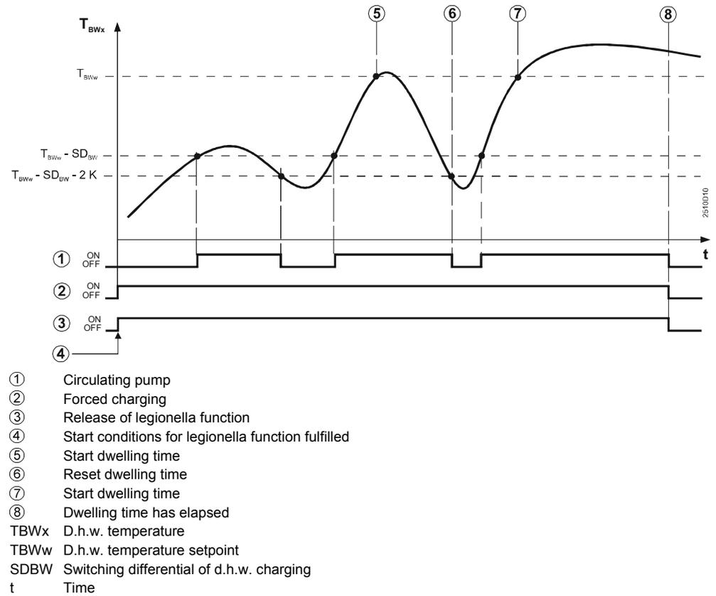
If set, a maximum d.h.w. charging time is also active here. If the legionella setpoint is not reached, the legionella function is interrupted to be resumed on completion of the maximum charging time.
