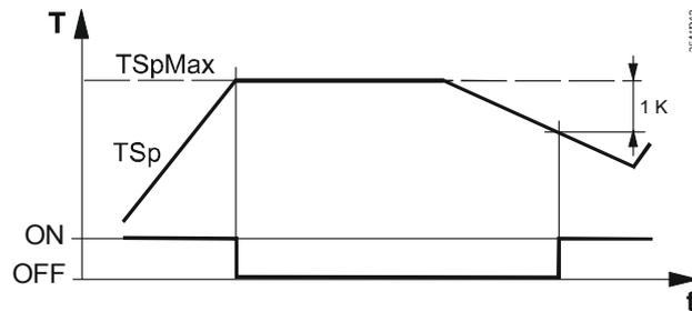
$T_{Sp}$  Storage tank temperature
