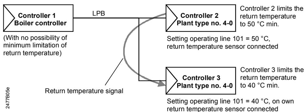
The zone controller with its own return temperature sensor (plant type 4 - x) passes the return temperature to the other zone controllers in the same segment. These can thus ensure minimum limitation of the return temperature locally, depending on the settings made, which means that they generate a critical locking signal internally. (For response to critical locking signals, refer to chapter 17.4.5 "Locking signal gain").
