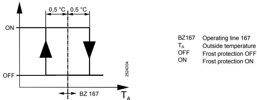
If the current outside temperature falls below the limit value (setting on operating line 167 minus 0.5 °C), the controller switches heating circuit pumps M2/M6 on and maintains the flow temperature at the setpoint selected for frost protection (operating line 168).
