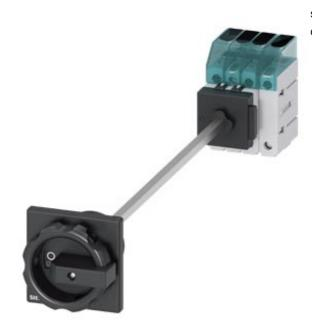
Load disconnector 3LD3, lu 16 A Main switch 3-pole + N Rated operating capacity at AC-23 A at 400V 7.5kW floor mounting Basic switch with door coupling Central hole mounting 22.5mm Rotating drive black  $66 \times 66 \text{ mm}$
