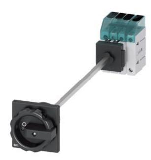
Load disconnector 3LD3, Iu 63 A Main switch 3-pole + N Rated operating capacity at AC-23 A at 400V 22.0 kW floor mounting Basic switch with door coupling Central hole mounting 22.5mm Rotating drive black  $66 \times 66 \text{ mm}$
