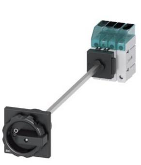
Load disconnector 3LD3, lu 32 A Main switch 3-pole + N Rated operating capacity for AC-23 A at 400V 11.5kW floor mounting Basic switch with door coupling Central hole mounting 22.5mm Rotating drive black 66 x 66 mm
