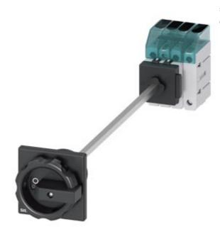
Load disconnector 3LD3, lu 25 A Main switch 3-pole + N Rated operating capacity at AC-23 A at 400V 9.0kW floor mounting Basic switch with door coupling Central hole mounting 22.5mm Rotating drive black  $66 \times 66 \text{ mm}$
