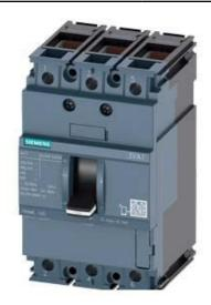
CIRCUIT BREAKER 3VA1 IEC FRAME 100 BREAKING CAPACITY CLASS S ICU=36KA @ 415 V 3-POLE, LINE PROTECTION TM210, FTFM, IN=16A OVERLOAD PROTECTION IR=16A FIXED SHORT CIRCUIT PROTECTION II=20 X IN CABLE CONNECTION
