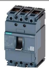
CIRCUIT BREAKER 3VA1 IEC FRAME 100 BREAKING CAPACITY CLASS S ICU=36KA @ 415 V 3-POLE, LINE PROTECTION TM210, FTFM, IN=40A OVERLOAD PROTECTION IR=40A FIXED SHORT CIRCUIT PROTECTION II=10 X IN BUSBAR CONNECTION
