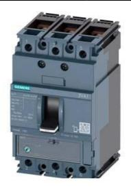
CIRCUIT BREAKER 3VA1 IEC FRAME 160 BREAKING CAPACITY CLASS M ICU=55KA @ 415 V 3-POLE, LINE PROTECTION TM220, ATFM, IN=20A OVERLOAD PROTECTION IR=14A ...20A SHORT CIRCUIT PROTECTION II=10 X IN BUSBAR CONNECTION
