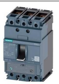
CIRCUIT BREAKER 3VA1 IEC FRAME 160 BREAKING CAPACITY CLASS N ICU=25KA @ 415 V 3-POLE, LINE PROTECTION TM240, ATAM, IN=50A OVERLOAD PROTECTION IR=35A ...50A SHORT CIRCUIT PROTECTION II=5...10 X IN BUSBAR CONNECTION
