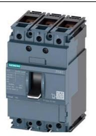
CIRCUIT BREAKER 3VA1 IEC FRAME 160 BREAKING CAPACITY CLASS S ICU=36KA @ 415 V 3-POLE, LINE PROTECTION TM210, FTFM, IN=63A OVERLOAD PROTECTION IR=63A FIXED SHORT CIRCUIT PROTECTION II=10 X IN BUSBAR CONNECTION
