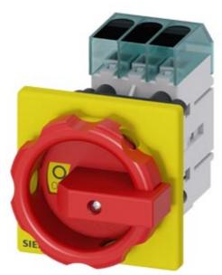
Load disconnector 3LD3, Iu 32 A Main switch 3-pole Rated operating capacity for AC-23 A at 400V 11.5kW Front plate mounting Basic switch with Central hole mounting 22.5mm Rotary actuator red / yellow 66 x 66 mm
