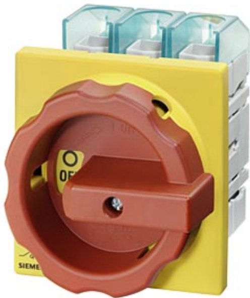
MAIN CONTROL SWITCH 3-POLE IU=125, P/AC-23A AT 400V=45KW FRONT MOUNTING FOUR- HOLE MOUNTING ROTARY ACTUATOR BLACK
