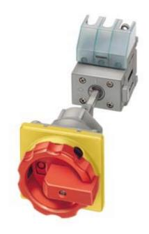
MAIN/EMERG. STOP SWITCH 3-POLE IU=100, P/AC-23A AT 400V=37KW FLOOR MOUNTING DIN RAIL/TWO-HOLE MOUNTING ROTARY ACTUATOR RED/YELLOW (EMERG. STOP)
