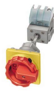
EMERG. STOP SWITCH 3-POLE IU=63, P/AC-23A AT 400V=22KW FLOOR MOUNTING DIN RAIL/TWO-HOLE MOUNTING ROTARY ACTUATOR RED/YELLOW (EMERG. STOP)
